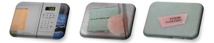
Place attached label in the flask in the desired location and cover with acrylic and press....trim...press...trim...place in compress and cure.
